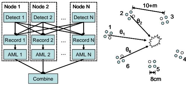
Figure 1: Block diagram of a DOA-based localization system.
