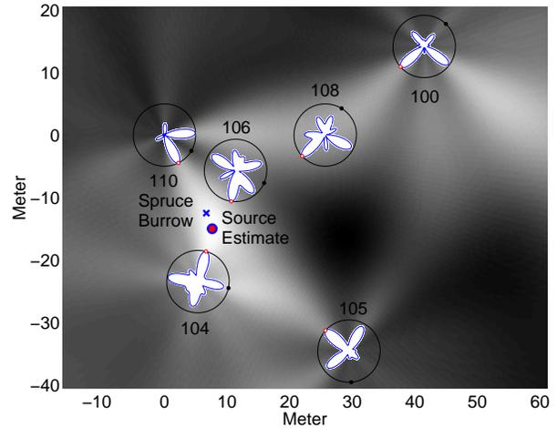
Figure 3: A pseudo-likelihood map generated based on the log-likelihood of all nodes, taken from the compact deployment. Main lobes are denoted by small dark gray circle on the log-likelihood ring. Black dots points to the array zero degrees.
