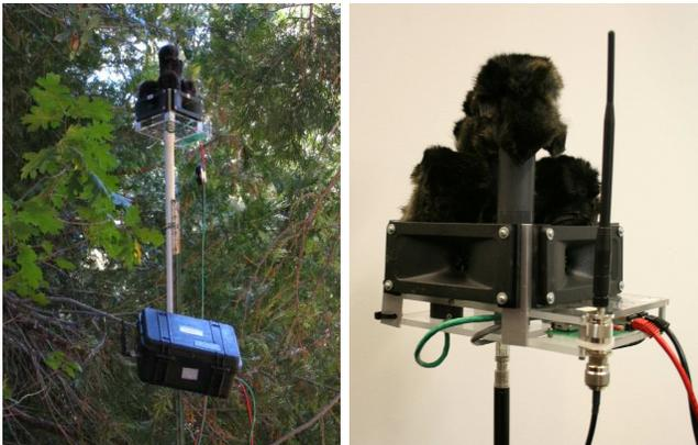
Figure 2: The Acoustic ENSBox Platform.
